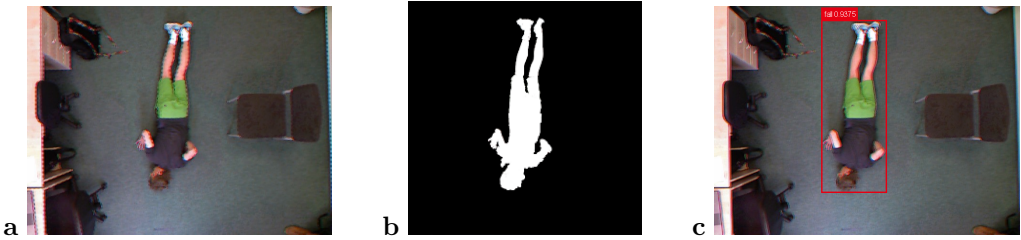
Fig. 7. Background segmentation in the preprocessing. (a) Original frame image; (b) reduced square segmented image; (c) final frame image with synthesized recognition box.
