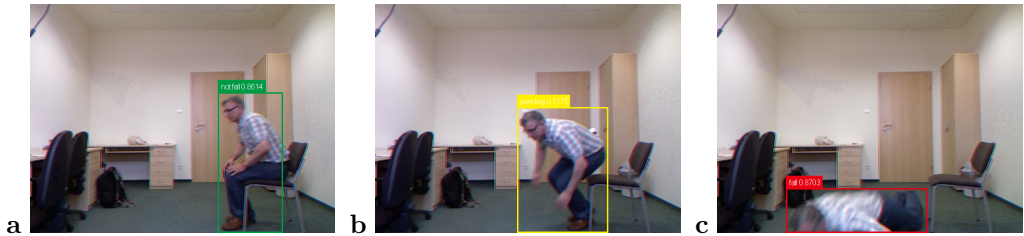
Fig. 8. Fall detection with 3D-SCNN. (a) Not fall; (b) pending; (c) fall.
