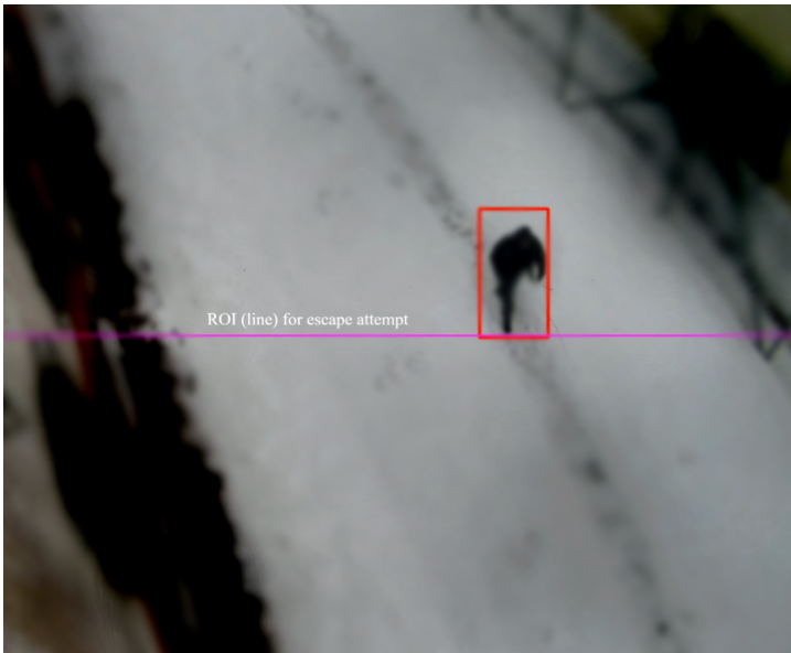
Fig. 7. Example of ROI line for detecting escape attempts outdoors and alarm notification.
