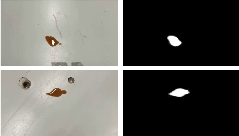
Fig. 2. Examples of visualised predictions that led to liquid detection and masks creation.
