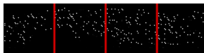
Fig. 8. Division of key points into four areas of equal width after applying RANSAC.
