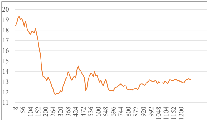
Fig. 10. Kernel Inception Distance graph for the micro dataset (500 images per class in the train subset) GAN training.
