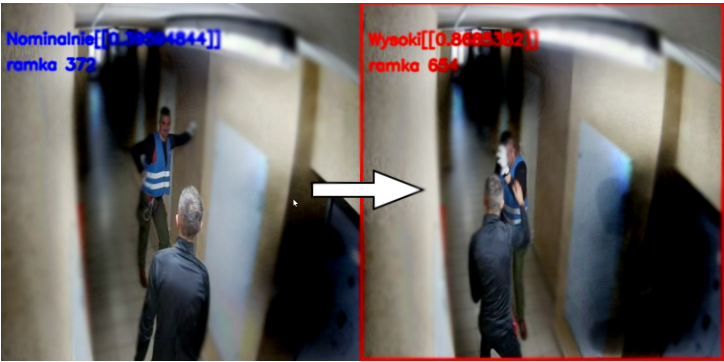
Fig. 6. Example of abnormal behaviour's detection and corresponding prediction value. Nominalnie – nominal; ramka – frame, Wysoki – high.
