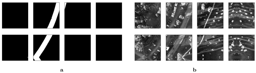
Fig. 5. Creating patches. (a) Patches from padded grayscale image; (b) patches from padded ground truth.
